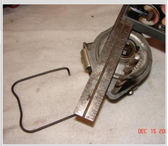
You can change points everyday & it will not fix bad bushings. If you are having trouble w/ points failure, check the shaft. If you detect movement, chances are it needs new bushings.
