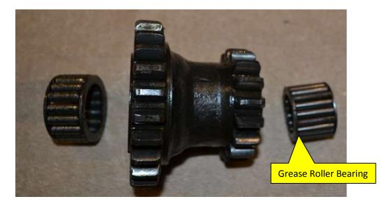
Don't forget to grease the cage bearings that are INSIDE the Idler Gear when you put it back together. The smaller one on the right is enclosed by the thrust washer and does not get much lubrication other than at initial assembly. There is a slinger slot on the end of the Idler Gear.
