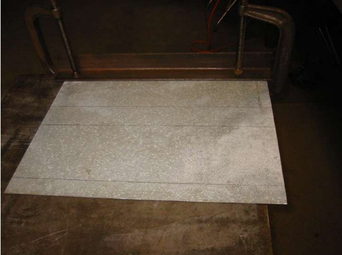
LAYOUT FOR FABRICATION OF NEW FUEL TANK,
