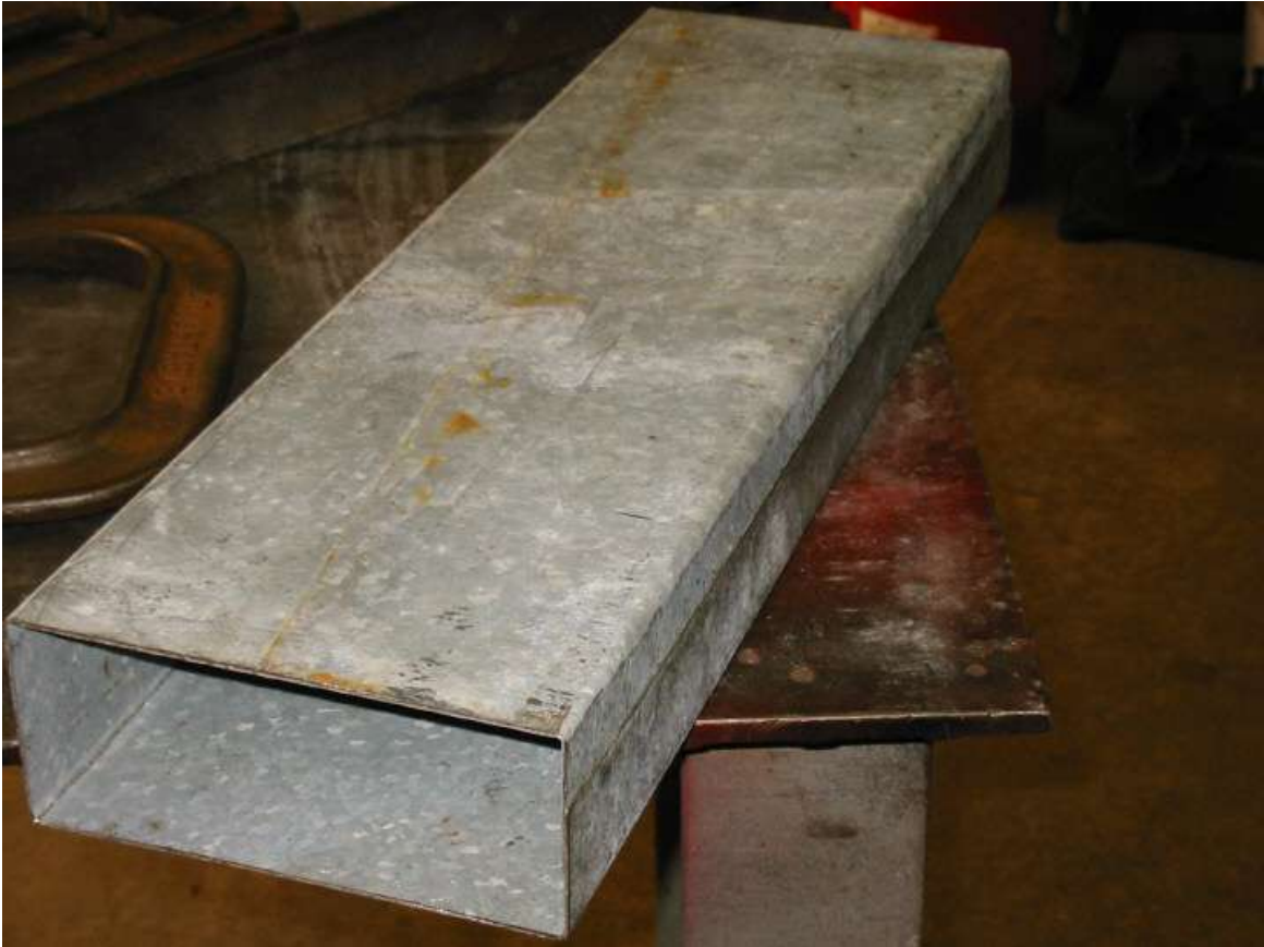
READY TO SOLDER ON THE ENDS
