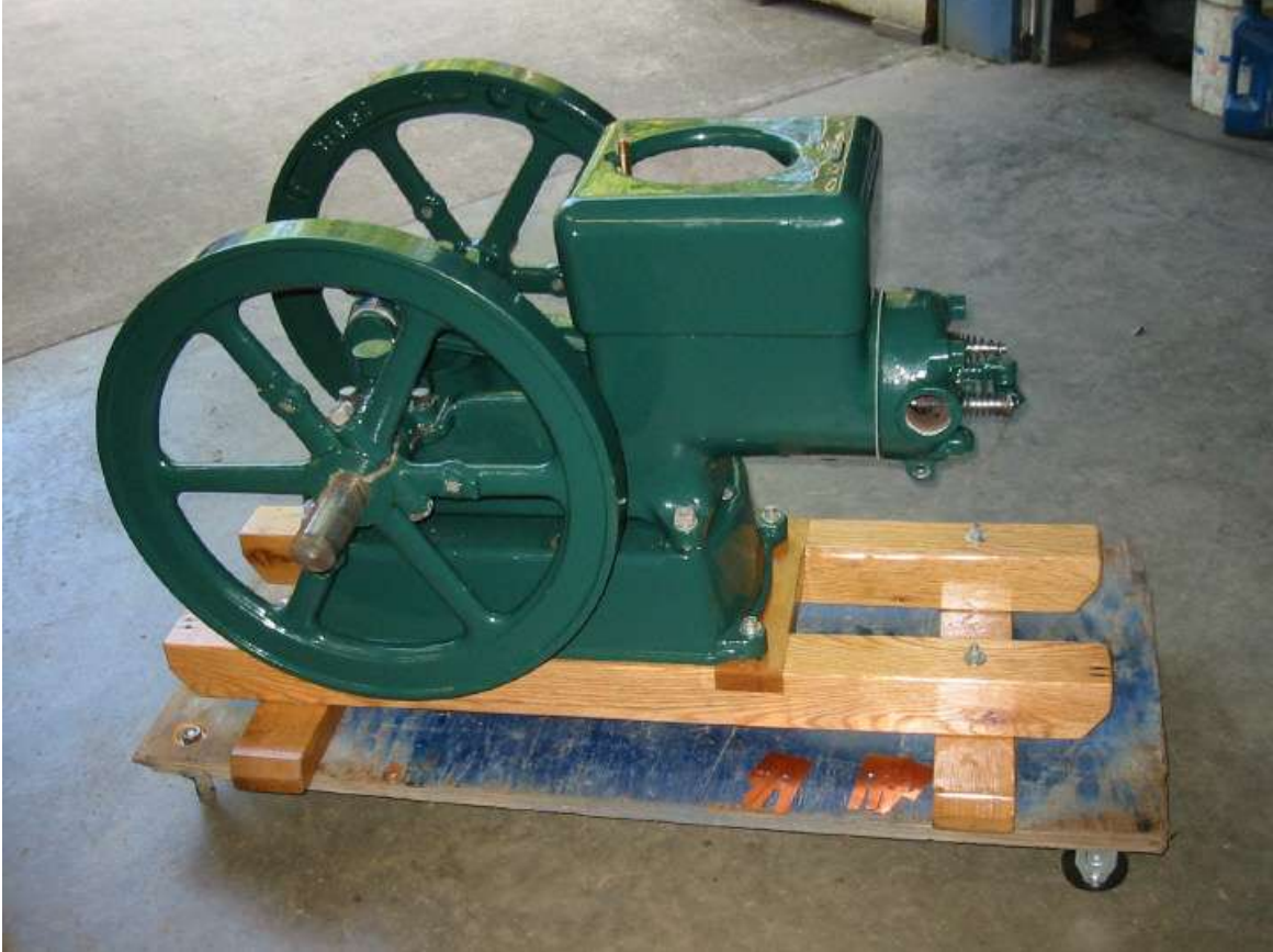
FINAL ASSEMBLY, FLYWHEELS, WATER HOPPER AND CYLINDER HEAD
